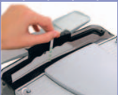
Dip the strip in water for 1 second. Check how many squares change colour.
